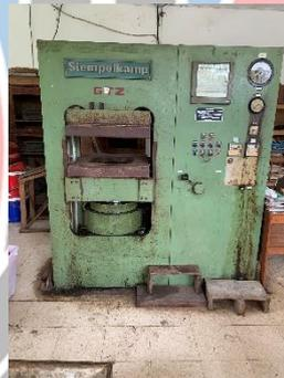
Gambar 3.8 Mesin *Compression Molding*
