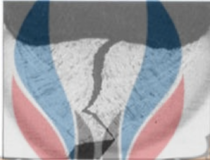
Gambar 2.7 Cold Cracking (Ramadhan, 2018)
