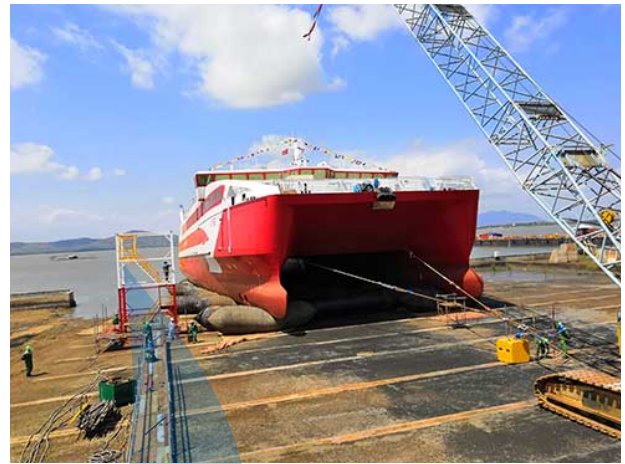
Gambar 2.3 Peluncuran End Launching Metode Airbag (Source, Google)
