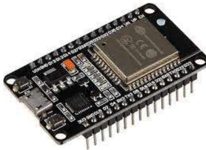
*Gambar 2. 1 Board Mikrokontroler ESP32*
