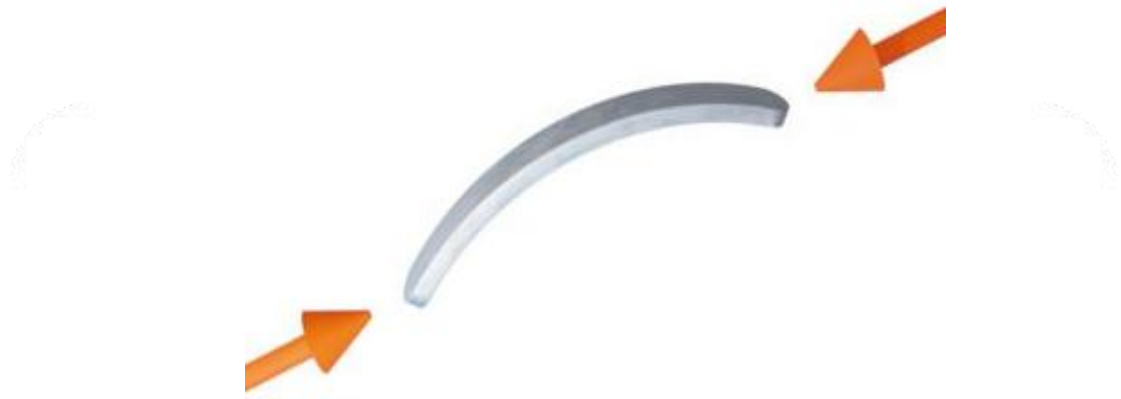
Gambar 2.1 buckling Failure (Sumber : https://efficientengineer.com )
