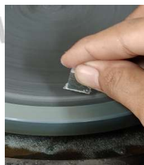
Gambar 3. 7 proses polishing paduan
