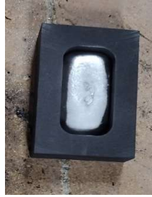
Gambar 3. 5 Proses air cooling
