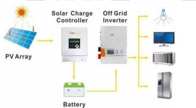
Gambar 2. 1 Diagram Prinsip Sistem PLTS Off-Grid (‘Buku PLTS.pdf’, no date)
