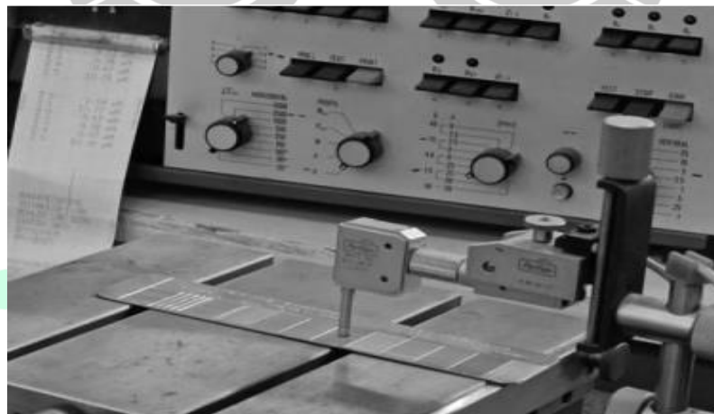
Gambar 2.7 Surface Roughness Stylus-type (Groover, 2013).
