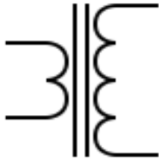
Gambar 2.4 Lambang Transformator Step Up
